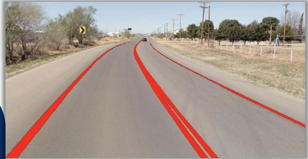
Pixel segmentation for paint striping identification.
